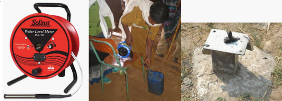
Figure 32 Dip meter (left), demonstrating use of a dip meter for the community in Dangila (middle) and monitoring well (right) established by IWMI (Barotse floodplain, Zambia). (Middle and right Photos: Alemseged Tamiru Haile).
