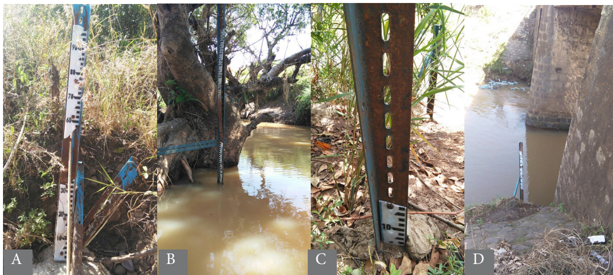
Figure 35 Broken, missing and corroded staff gauges installed at a) Deme at OretaAlem, b) Rebu River Nr. Wolkite, c) Wabe River Nr. Wolkite and d) Darge River Nr. Tedelle (Source: IWMI unpublished report).
