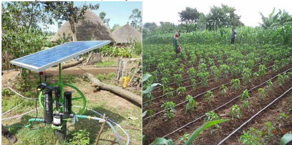
Figure 9. Solar pump linked to drip system in central rift valley (Photo credit: Amare Hailelassie).
