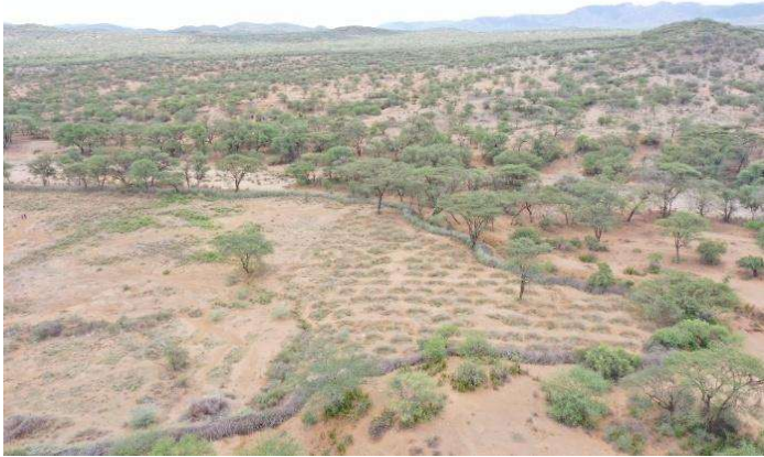
Half-moon water harvesting structures slow runoff, increase infiltration and soil moisture, and support vegetation recovery in degraded rangelands. Lokiriama, Turkana County, Kenya. Photo credit: Stephen Mureithi and Aida Bargaés Tobella (Restore4More).
